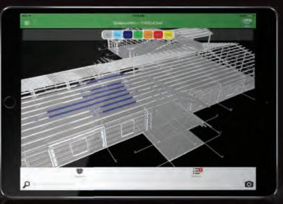
STATUS MODE | Color code each part to tag status as received, staged, installed, missing, damaged or unused. Statuses are uploaded automatically when connected to the Internet.
