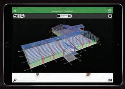
**BUILDING GRIDLINES** | Gridlines are displayed as an overlay with the 3D building model, providing a method of orientation and direction on-screen. These allow you to quickly orient yourself with the building layout and easily identify where your parts need to be placed.
