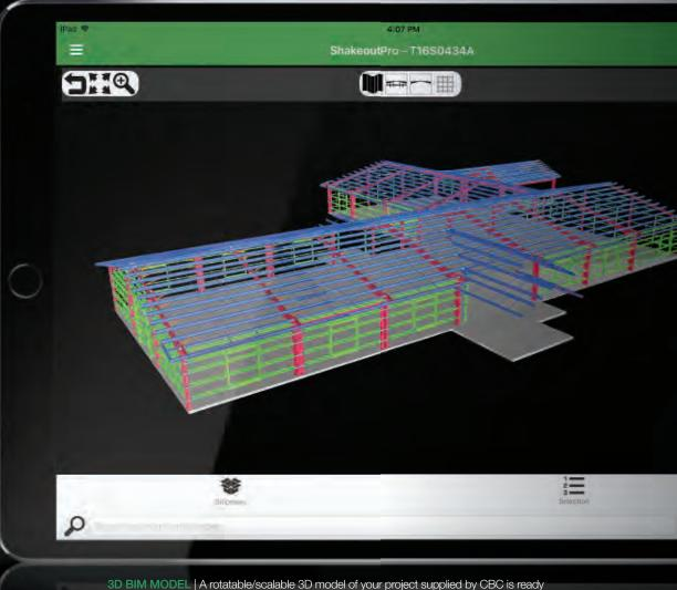
3D BIM MODEL | A rotatable/scalable 3D model of your project supplied by CBC is ready to be rendered to your device screen. View your project on-screen before unloading it on-site.
