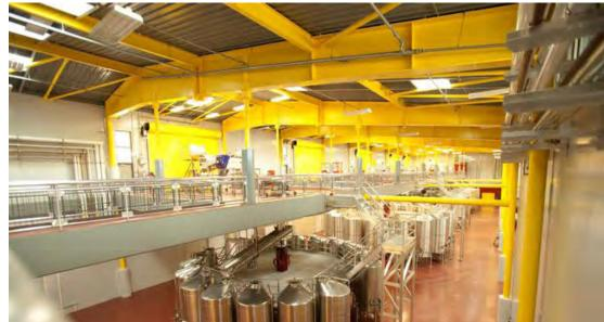
Construction of this 60,00 square-foot state of the art winery production facility; utilizing Hybrid building system including insulated concrete walls, with CBC Primary and Secondary Framing systems and RD-5 roof panels. This project was awarded LEED Silver Certification.
