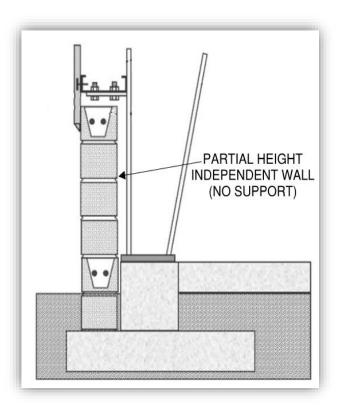
to be designed for additional loads from the CBC wall panel depending on the transition details.
