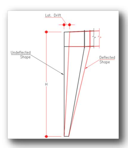
Figure 1 - Frame Lateral Drift (sidesway)
