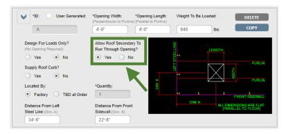
The first detail to look at is the weight of your RTU. CBC's guidance requires that any RTU weighing more than 1,000 lbs. should have independent framing members. These members are usually built-up or hot rolled beams used to support the heavier RTU loads. This type of framing requires purlins to be cut, so there is little benefit for allowing purlins to run through the opening.
